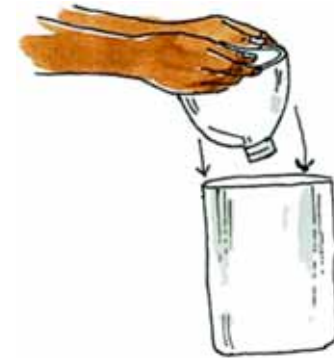
3. Insert and glue the reversed upper part of the bottle into the bottom part
